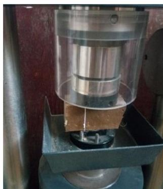
**Figure I.30-** Essai de compression
